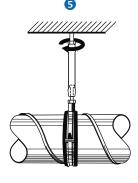
\*Optionally, the pipe, the pipe clamp and the adjustment element can already be pre-assembled in step 1.
